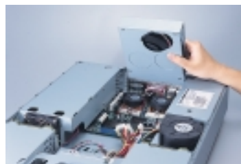
Fan tray for better CPU heat dissipation
